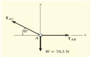
$T_{AB} = k_{AB} s_{AB}; 136.0N = 300N/m(s_{AB})$   $s_{AB} = 0.453m$ For stretched length,  $I_{AB} = I'_{AB} + s_{AB}$   $I_{AB} = 0.4m + 0.453m$ = 0.853m
