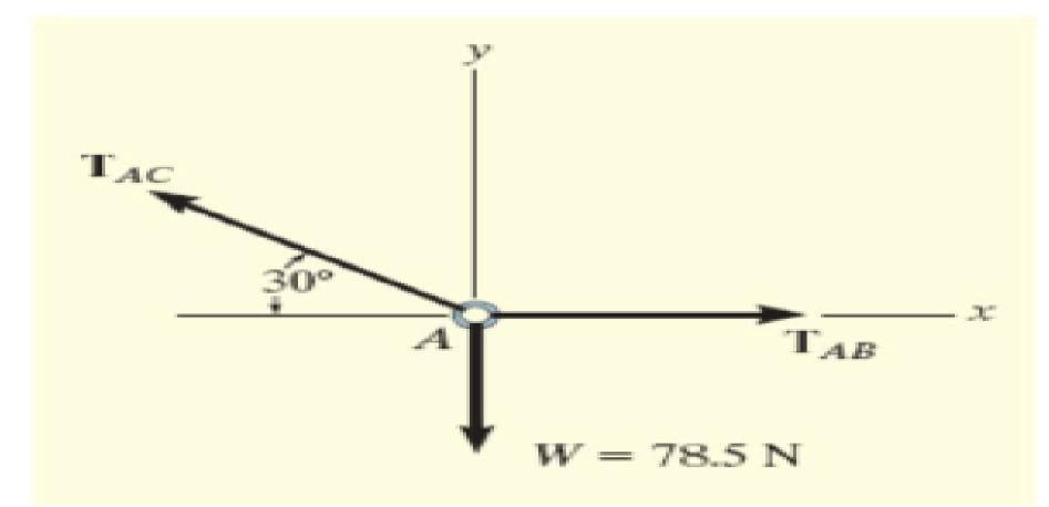
+→  $\sum F_x = 0; \quad T_{AB} - T_{AC} \cos 30^\circ = 0$ +↑  $\sum F_y = 0; \quad T_{AB} \sin 30^\circ - 78.5N = 0$ Solving,  $T_{AC} = 157.0$ kN  $T_{AB} = 136.0$ kN
